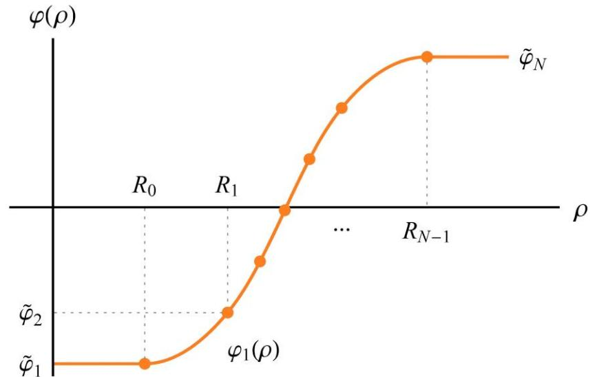
$$V_s(\varphi) = \underbrace{\left( \frac{\tilde{V}_{s+1} - \tilde{V}_s}{\tilde{\varphi}_{s+1} - \tilde{\varphi}_s} \right)}_{8 a_s} (\varphi - \tilde{\varphi}_s) + \tilde{V}_s - \tilde{V}_N.$$
