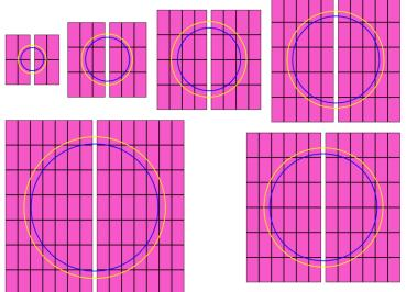
Approximately 6 layers with 400 ALPIDE sensors. Basically geometry of SAVD with additional sensors and layers.
