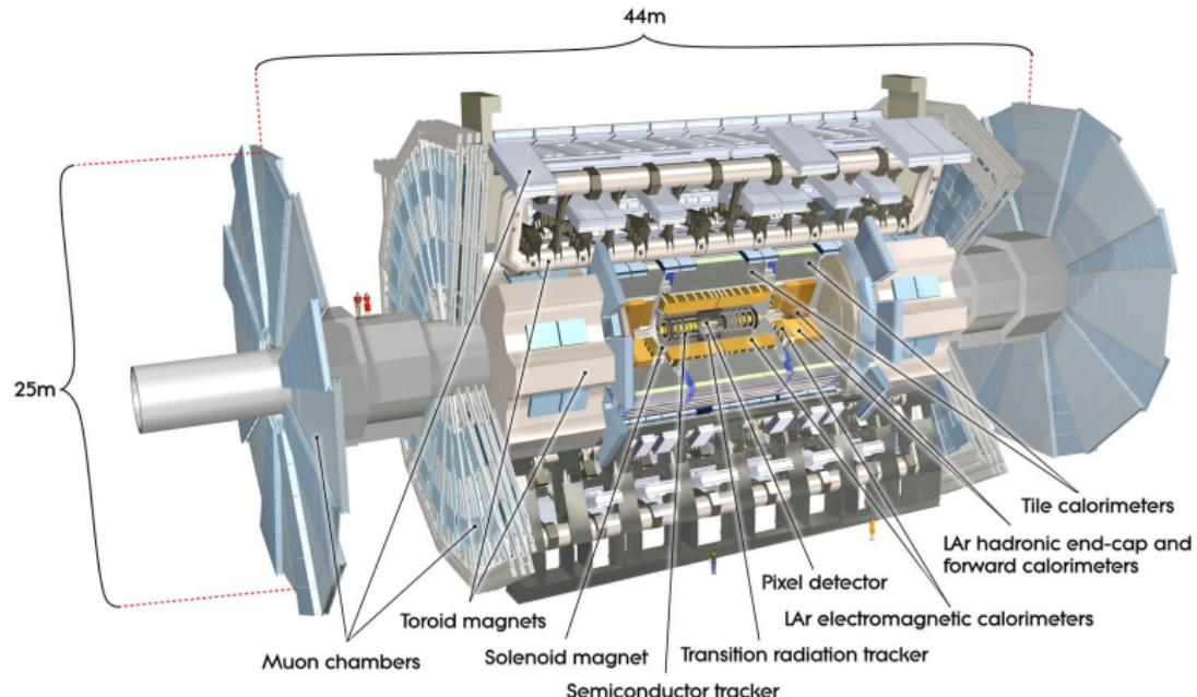
...but also forward detectors providing measurements
