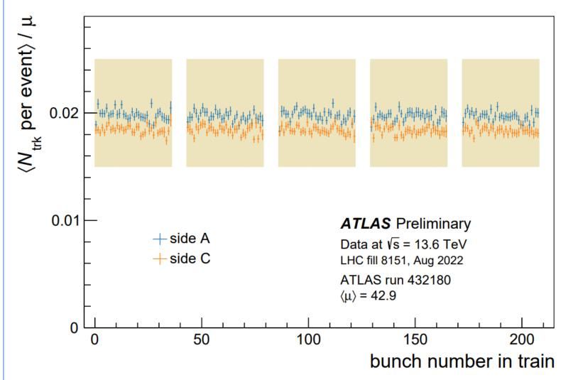
Average track multiplicity on the given side in dependence on the bunch number in train weighted by pile-up at that train. No dependence on bunch number in train is visible which indicates none or very small dead-time effect.
