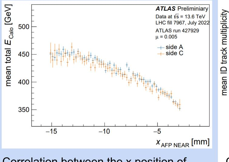
Correlation between the x position of reconstructed tracks in AFP NEAR stations and the total energy measured by the ATLAS Calorimeters for side A and C.
